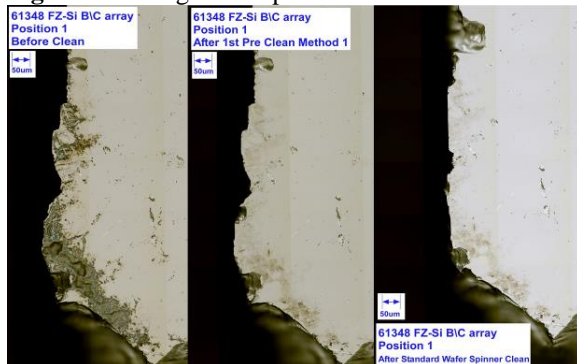
Figure 6: Before and After Cleaning of Position 1
